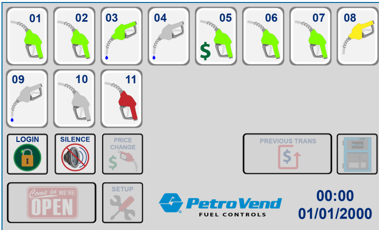
Initial Main Screen Online with Pump Status
